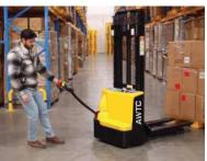
When truck is down, release the brake to move the unit manually.
